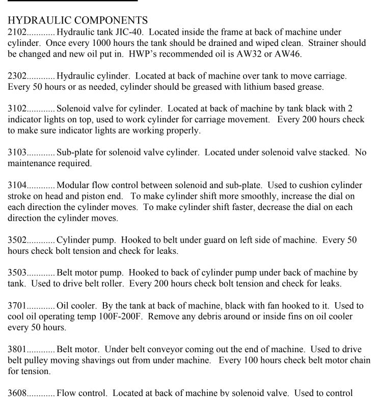
speed of carriage. Every 200 hours check bolt tension and for leaks.
